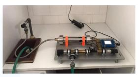
A device developed by researchers to measure the effect of IPS-treated water at different pressures on plant growth.
